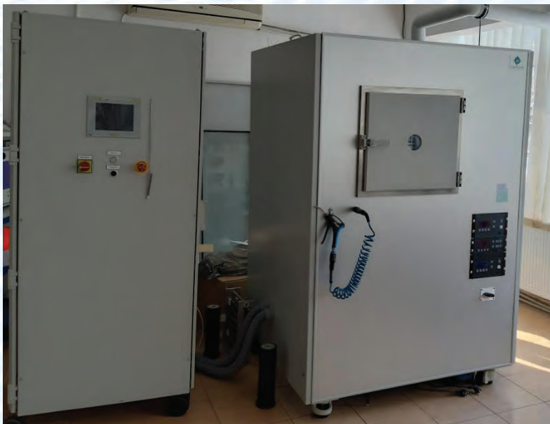
Fig. 51. – Instalatie de plasma tip 400 CD Roll-to-roll (Furnizor Europlasma Belgium)
